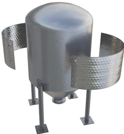
Lift each clamp-on section into its designated place on the receiving equipment. Verify that the section(s) have proper clearance around all outer edges (Recommended 1/2" clearance minimum). It is important to remember that each clamp-on section will thermally expand and contract during operation and any interference in this movement of the clamp-on section(s) could cause damage or performance losses.
